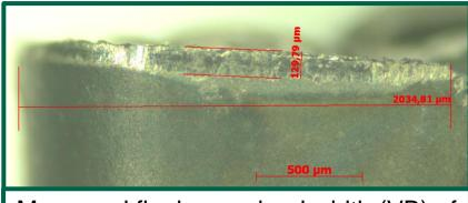
Measured flank wear land width (VB) of major cutting edge after both final rough and finish cuts using microscope
