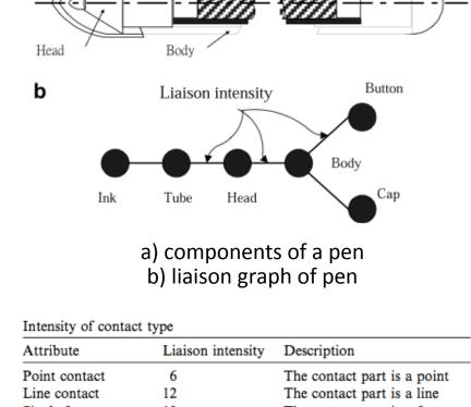
Single face contact The contact part is a face Many points will be contacted Multi-point contact Many faces will be contacted Multi-face contact Example of CT liaison intensity scale
